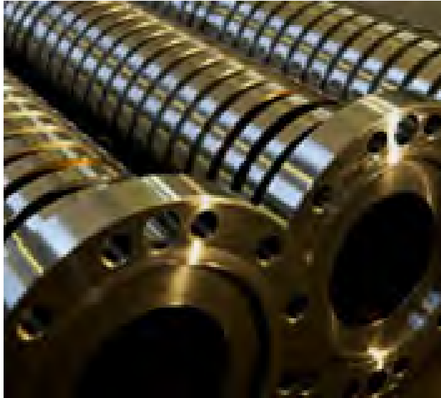
Fig. 25. Extruder screw, Cronidur 30 [ETE-11].
