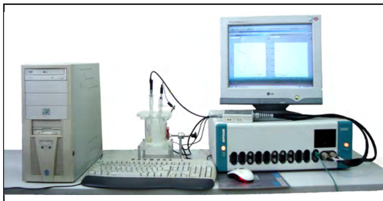
Fig. 3. The set of appliances for the electrochemical corrosion testing by EIS technique.
