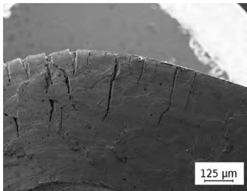
Fig. 25. Deep corrosion cracks in 25Mn-3Si-1.5Al-Nb-Ti steel after bending and the immersion in 3.5wt% NaCl.
